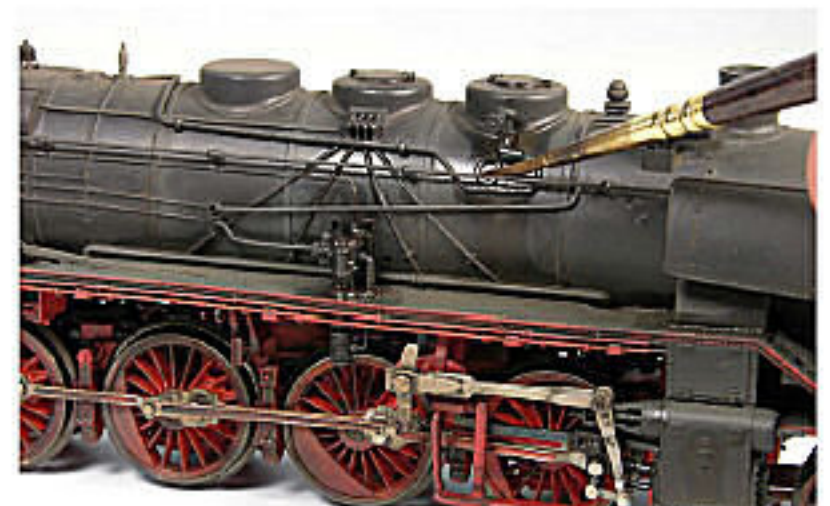
Using a brown enamel wash, we will create some streaking grime and rust staining.
