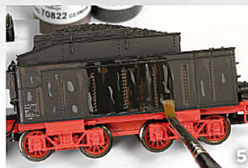
Now we dampen the surface with the alcohol.
