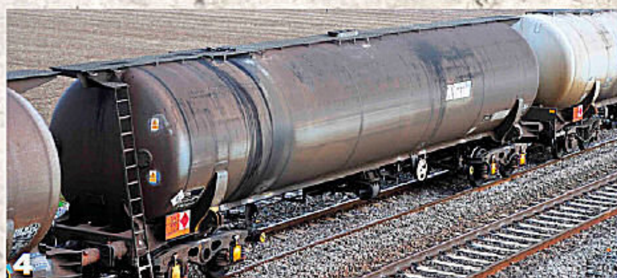
4 More scratches along the sides. The spilled oil on this wagon has run down the sides in thin lines instead of large stains.
