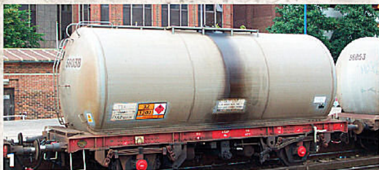
1 Here is a classic example of the oil staining on the side of one of these oiltanks. Notice how clean the wheel hub covers are.
