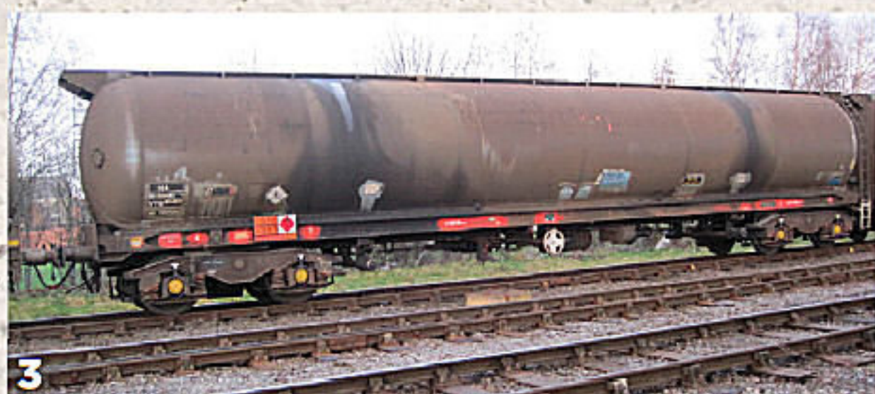
3 In this example we can see how all the information and warning labels have been kept clean and free from grime.
